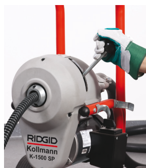
Engage clutch, cable spins
